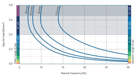
Natural frequency of a single-degree-offreedom system consisting of a fixed mass and an elastic bearing consisting of VIKFOAM VF 400 on a stiff subgrade.
