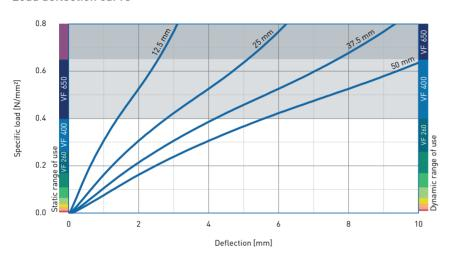
Recording of the 3rd loading; testing between steel plates at room temperature measured with a deflection rate of 1% of the thickness per second
